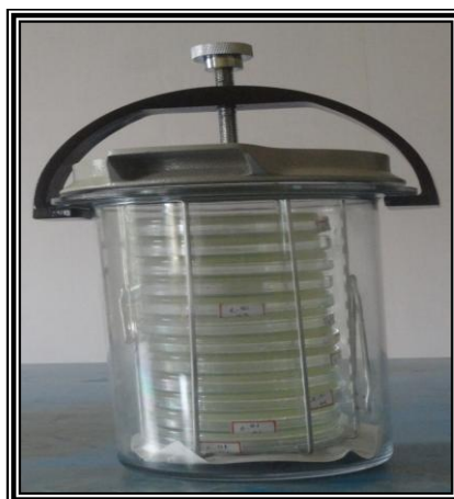
Figure 2: Gas pack method for anaerobic bacteria
